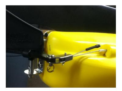
Sit inside your Journey and test motion of all of the rudder components. If the cables feel like they stick, try some spray silicone in the tubes.
