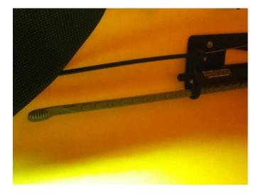
Place the Mini Clam Cleat found in the Rudder Housing Packet into the slot on the Starboard outside side of the boat in front of where the ¼" Black Tubing comes out of the hull. Mark the holes for the screws and drill out with a 1/16" drill bit. Install the Clam Cleat using the small bolts and nuts supplied in the Rudder Housing Packet.
